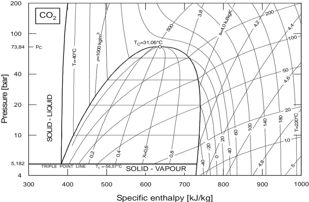
Figure 1 – Thermodynamic diagram *specific enthalpy – pressure* for Carbon Dioxide.
