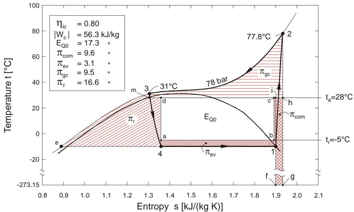
Figure 3 – Exergy losses  $\pi$  depicted in a  $T$ - $s$  diagram for  $\text{CO}_2$ , relative to a simple transcritical refrigerating cycle.
