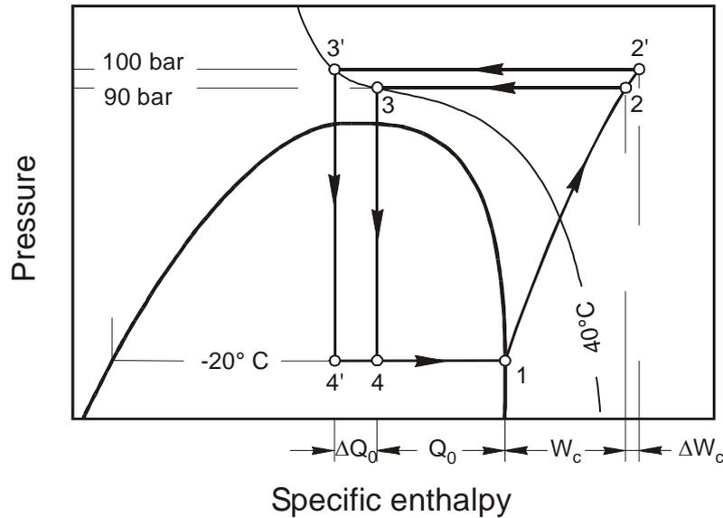
Figure 2 – Two transcritical refrigerating cycles (with different values for the gas cooler pressure) depicted in the *h-p* diagram for CO<sub>2</sub>.
