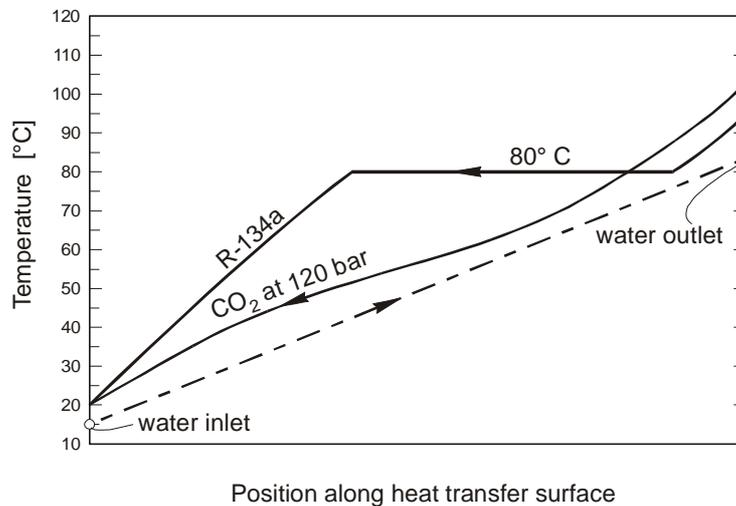
Figure 5 – Temperature profiles in transcritical CO<sub>2</sub> heat pump gas cooler, and in a R-22 heat pump condenser, to heat water from 15 to 84 °C.
