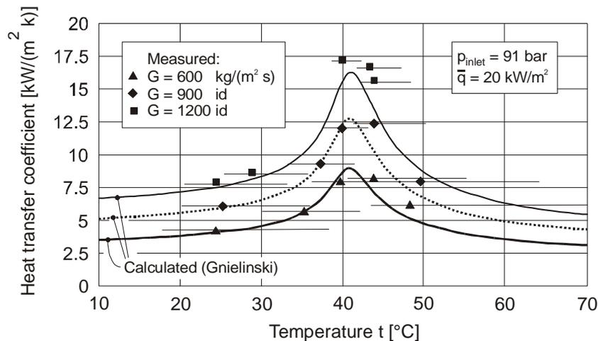
Figure 4 – Influence of varying mass flux on the supercritical pressure heat transfer coefficient, in a microchannel aluminium tube with 25 circular channels with 0.79 mm inner diameter (Pettersen and Vestbøstad 2000).
