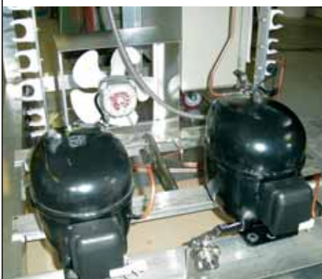
Figure 2. Detail of the double compressor unit of the test rig TWIN-CO 2 .
