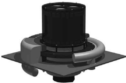
Fig. 2. The design of a prototype developed in the Thermal Science Institute of the University of Applied Sciences of Western Switzerland. This machine is based on the rotation principle. The magnets may be seen on the left back 180°. The front right side contains no magnet assembly and, therefore, yields the region with no magnetic field. Tubes for the heat transfer fluids are shown. In the cylinder above the magnetocaloric ring a motor to drive the refrigerator is assembled.
