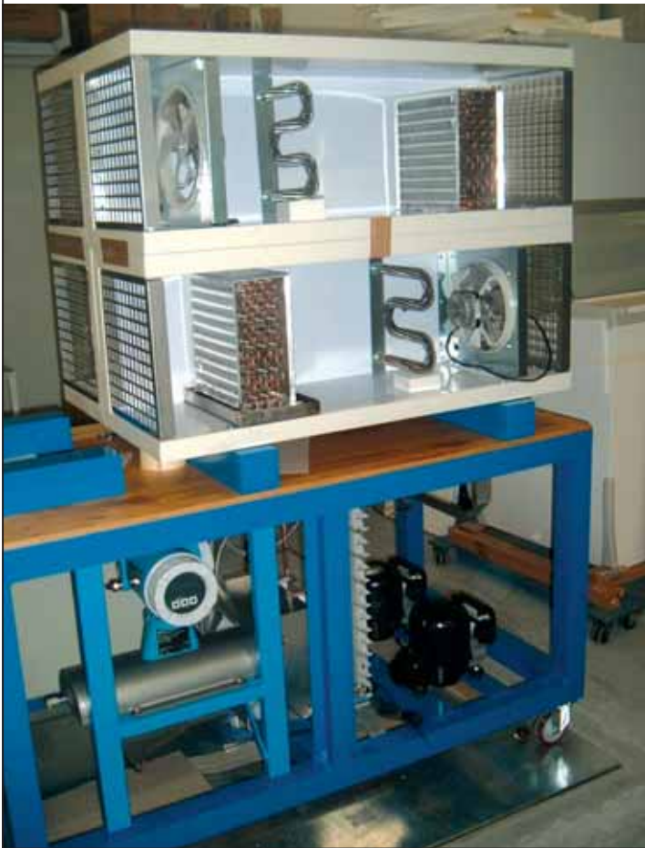
Figure 2. Detail of the double compressor unit of the test rig TWIN-CO 2 .
